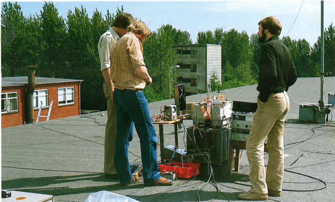
The SKANTI antenna tuner is tested under realistic conditions. Here on the roof of the main building in Værløse.
