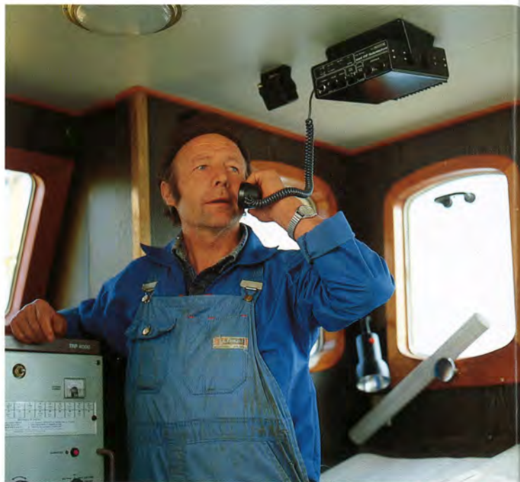
A TRP 4000 and a VHF 2500 radio telephone being used in the wheel house of a fishing vessel.
