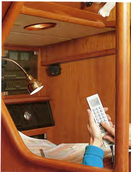
The compact two-unit design of the VHF 3000 was made possible by the use of Surface Mounting Technology.
