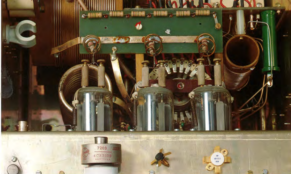
The transmitter valves in a TRP 400. On the metal strip at the bottom of the picture are some of the later-generation components: left, the ceramic transmitter valve used in the TRP 5000; centre, the transistor used in the Marinetta TRP 1; right, the transistor used in the TRP 8000 in 1983.
